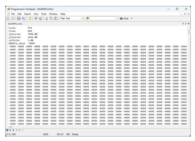
The data a whole load of elevations in a grid. The first few lines of the data file tell us the coordinates of the origin of the grid and the grid interval.
