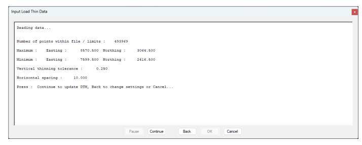
Even with such a fine vertical tolerance – in this case of only 1cm, the thinning has reduced the points down to 25,498. Bear in mind that this particular dataset only had an accuracy at best of +/- 5cm anyway, so allowing a further +/- 1cm isn't a problem.
