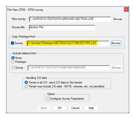
LSS will automatically specify the new filename, based on the load file you created during the plot. Change the Prototype survey to be the "Section Plot Prototype.LSS" as shown above.
