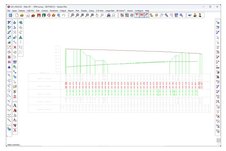
To create the DXF, go to "Export / AutoCAD DXF" and specify the name of the DXF you want to create. Then unless you have any specific layernames specified in an AutoCAD Description File (ADF), the leave all the options as they are.
