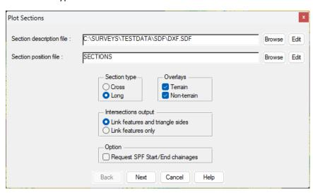
It is suggested that you use the Section Description File "DXF.SDF" if you are intending on just plotting the section to DXF and are not concerned with border / title block details. The DXF.SDF will plot all the sections on one large sheet.
