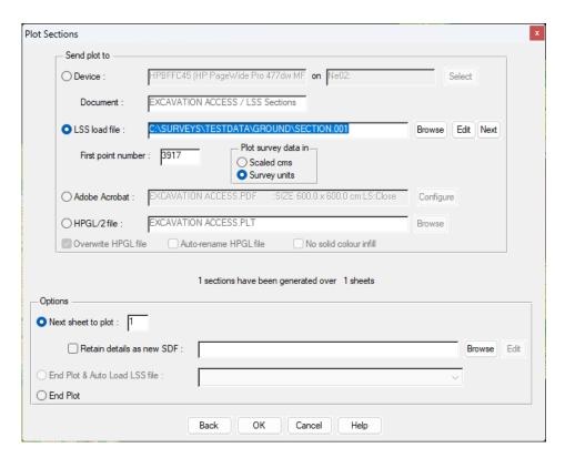
Choose the option "LSS Load File" and type in a load file name. At this stage you will need to decide whether the final DXF file is to be in "Survey Units" (i.e. Metres) or "Scaled Cms" (plotter centimetres). If you choose the former, the vertical and horizontal scales (as specified when the SPF was originally created) will have to be the same.
