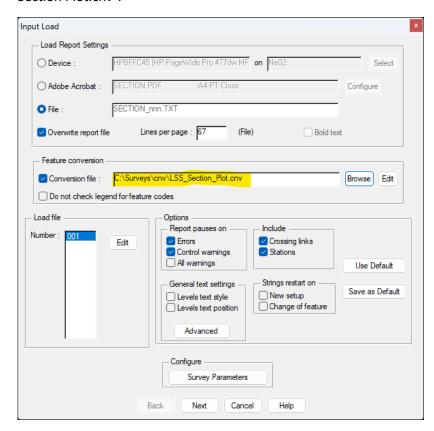
Follow the on-screen prompts to generate the LSS survey containing your sections. When it first appears, you may only see dots, especially if there are a large number of section plotted. You can go to "Configure / Display Controls" and increase the "Dot mode when screen > " value.
