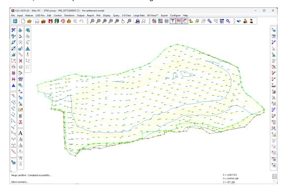
You should see that the contours will change accordingly, to represent the change in levels for the pre-settlement adjustment.
