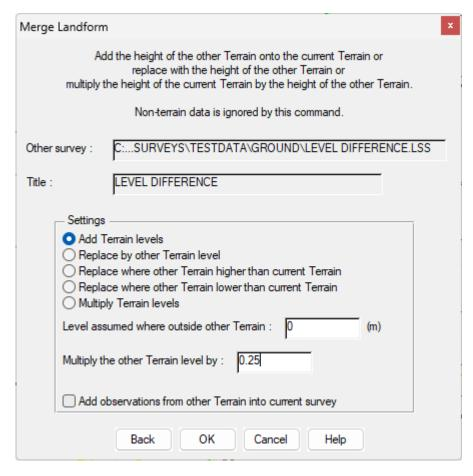
Here we need to "Add Terrain levels" from the level difference model, but also to "Multiple the other Terrain levels" by a specific value. This value is key to how this command works.
