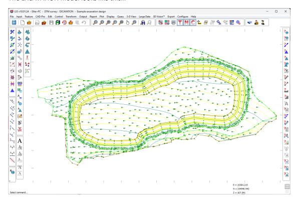
We will create the level difference for the entire survey, and include observations from BOTH models. We will also ensure that the level difference is positive where the current survey is above the other.
