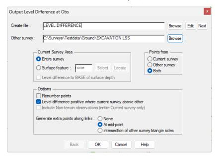
Here we are going to create a model called "LEVEL DIFFERENCE.LSS", where each point in both surveys will be the level difference between GROUNG and EXCAVATION.
