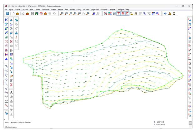
As this is representing the restoration design, we need to alter this model to represent the pre-settlement levels. So first we need to SaveAs under a new name. So we go to "File / Save As" and call it "PRE-SETTLEMENT"
