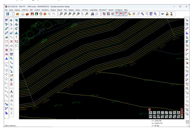
Create a section position file. Choose section interval and offsets.
