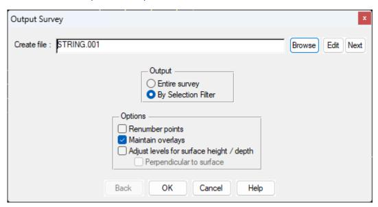
Here we can select the option "By Selection Filter", as this will enable us to only output selected points from the survey.
