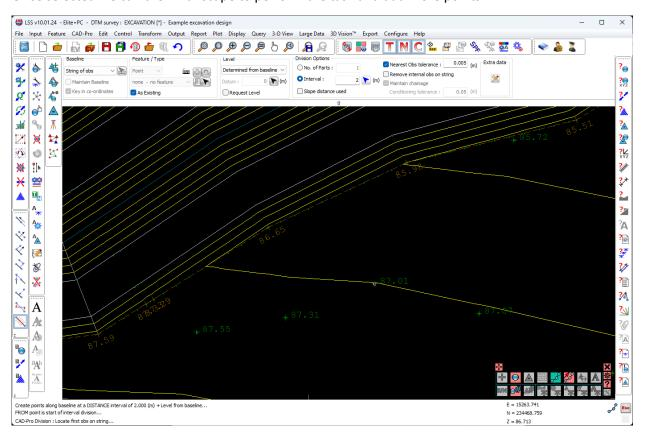
Now we need to output selected points to a new LSS load file. So we select the command "Output / Survey"
