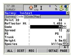
To amend your display mask to match that shown above choose **Management / Configuration Sets** from the main menu. Highlight the configuration set to be updated then select **New** to create a copy of this config set (select **[F3] Edit** to change the existing one) typing in the new **Name** and **Description** etc. Click **Store** to create the copy.
