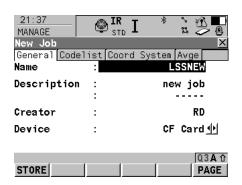
Returning to the Survey Begin page, the *Coord System, Codelist* and *Config Set* should be set for the new survey e.g. as per the LSS media 'Support\_files' folder.
