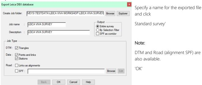
LSS will export the *entire survey* into the necessary DBX files which are copied onto the instrument card job folder via the card reader.
