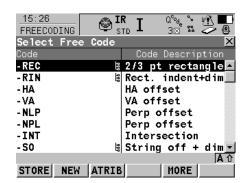
A Free-code applies to 'One shot' only as it only applies to the current observation and does not appear on subsequent measurements.
